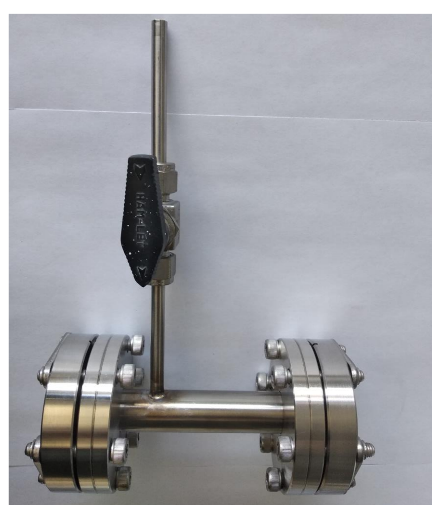
Sample holder for UV-Vis transmission measurement under vacuums
